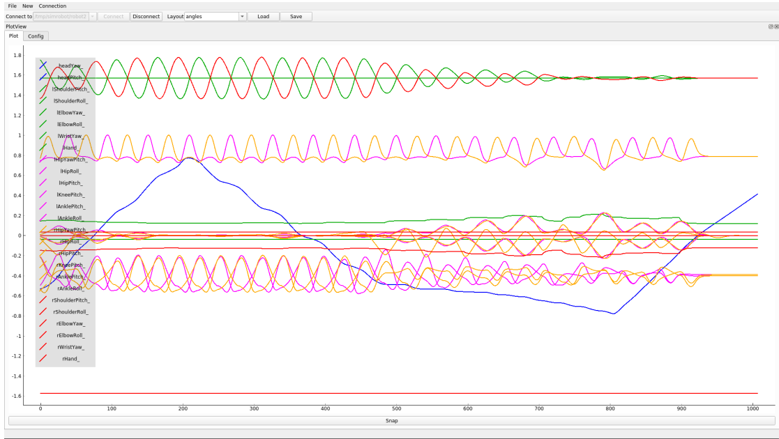
Figure 7.3: A Plot-panel showing all joint angles.
