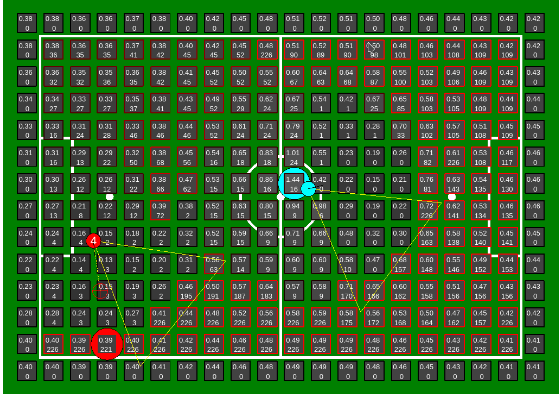
Figure 5.10: This is a visualization of the ball search map. The probability (upper value inside the cells) is represented by the brightness of the cells while the age (second value inside the cells) is represented by the red border. Also the players with their field of view and current target cell are visualized.
