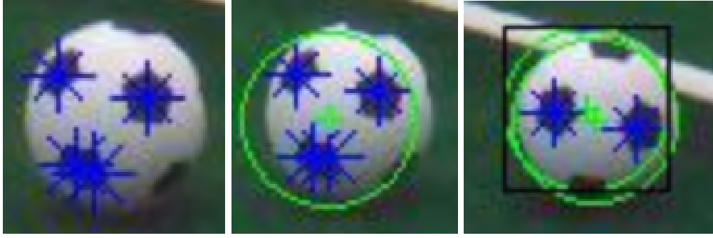
(a) Seed points corresponding to the center of the black patches on the ball. (b) Merged seeds and projection of the corresponding ball radius. (c) Reprojected ball from result of the ball filter (green circle within black rectangle).
