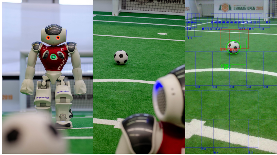
Figure 1: NAO robot in a ball detection situation. On the left, NAO robot with its two cameras in the head. In the middle, a ball from the robots perspective. On the right, an image from the robot’s camera augmented with debug information about the ball detection.
